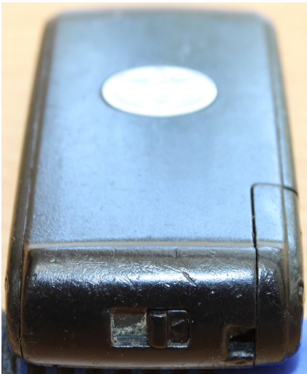
Hook of sliding latch knob at top of key remote
